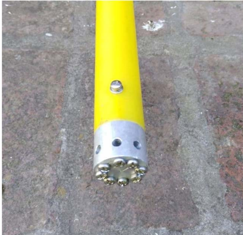
Photograph 1.- Detail of the support piece of the rods that make up the electrode.
