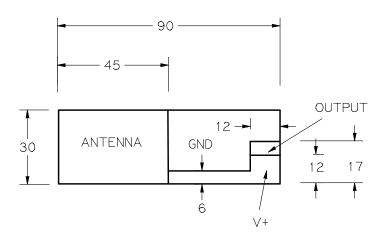
The traces are cut using a Dremel tool.
