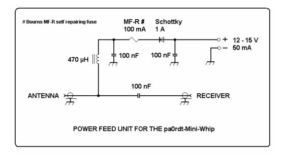
Power is fed to the *pa0rdt-Mini-Whip* via the coaxial feed line. A Power Feed unit couples the power trough the coaxial feed line to the *pa0rdt-Mini-Whip*. A second coaxial cable couples the signal to the receiver.
